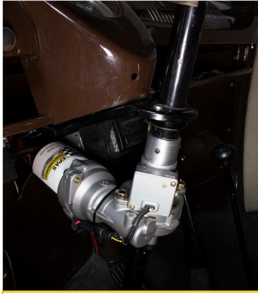
Align the woodruff key hole at 12 o'clock position while installing the motor onto the lower steering shaft.
