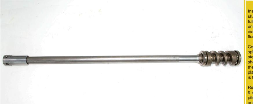
Install the splined steering shaft (insuring the shaft is fully seating inside the motor end) and weld in place, insuring that the weld is flush with the coupler.
